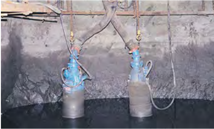
: Slimline Pumps - Pump diameter less than 15"
